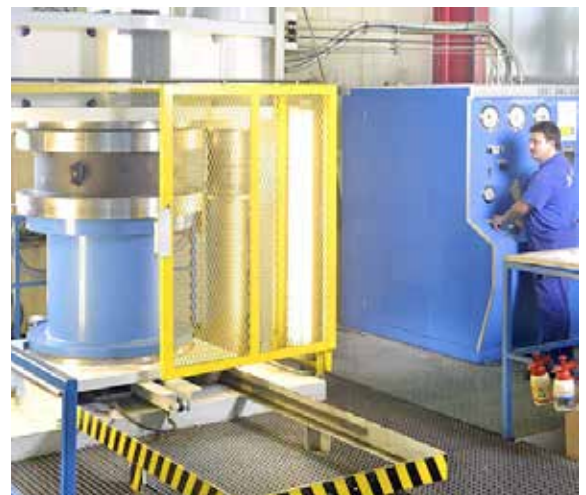
Hydraulic/Pneumatic pressure test bench
