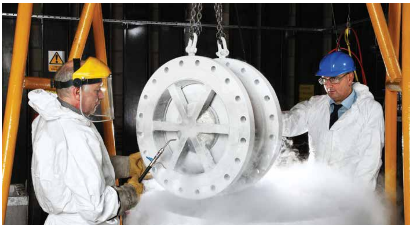
18" 300# Nozzle Check Valve Type NKF on Cryogenic Test
