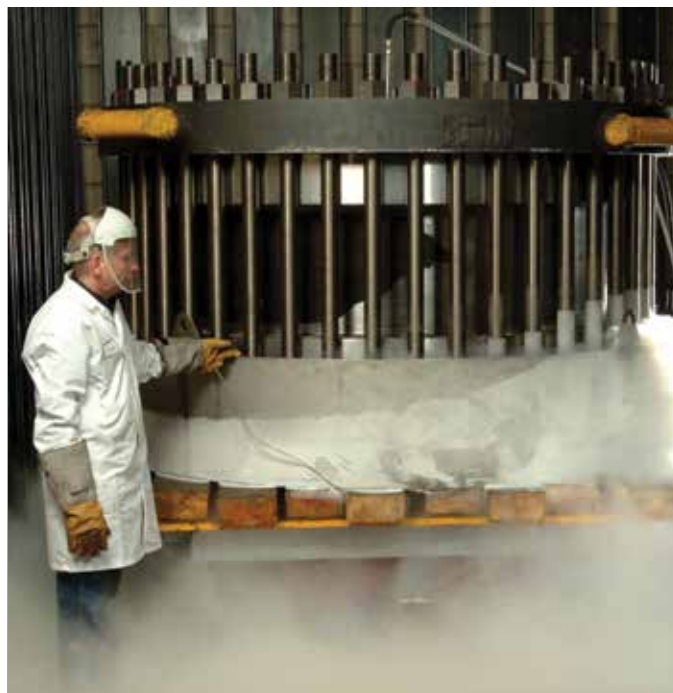
Cryogenic test facility for helium leak testing
